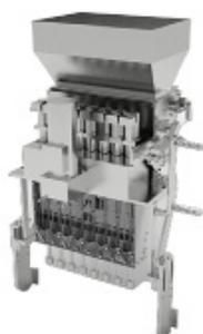
*auger filling system for powders*
