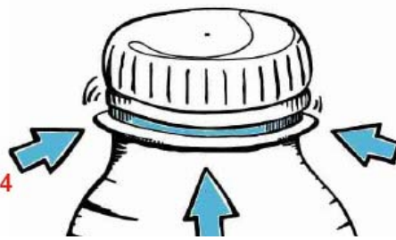
Front view apparently ok but bad cap seat at opposite side
