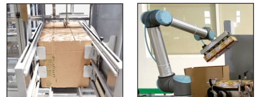
Integrated case erector with case packer
